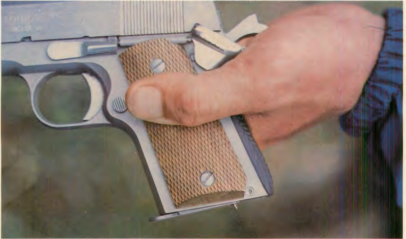
ABOVE: Fully loaded indicator protrudes from bottom of magazine to indicate weapon's status to shooter.
